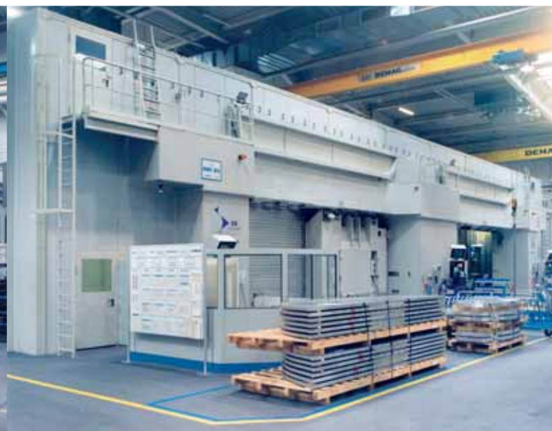
Also machines of type ACM are in use at Airbus Varel. Operators and manufacturer are convinced that this is the largest four-spindle machining center in Europe.
