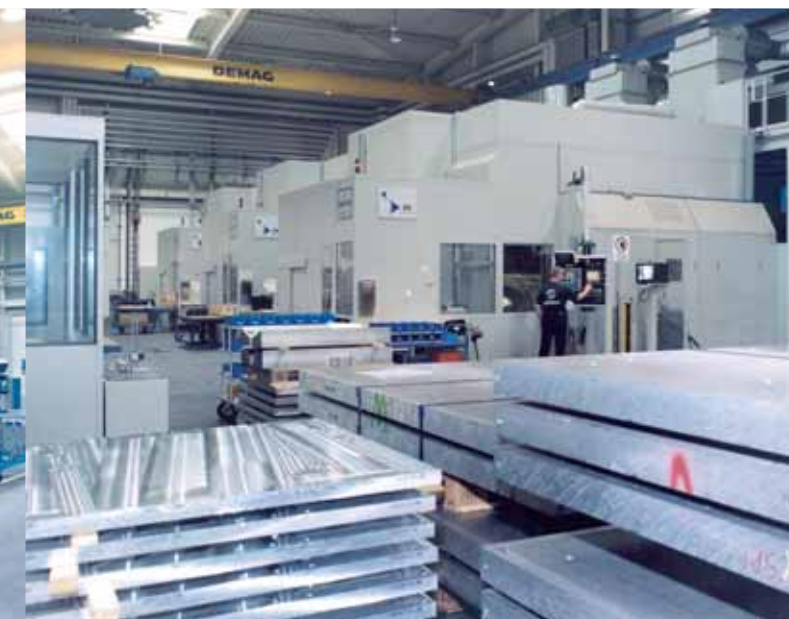
The three ECOSPEED 2500 operate in a linked arrangement, with two load - unload stations and six buffers.
