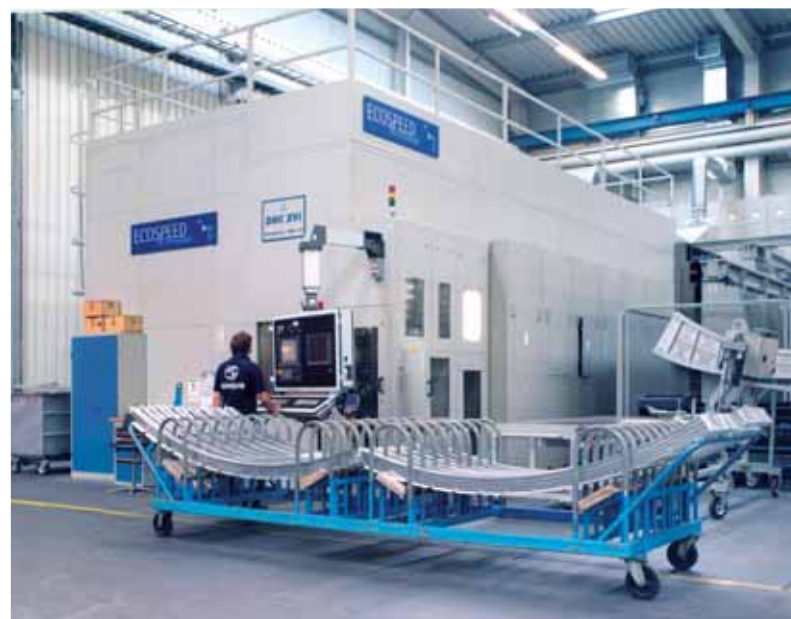
ECOSPEED 2600 process aircraft structural parts up to 7,000 mm in length.
