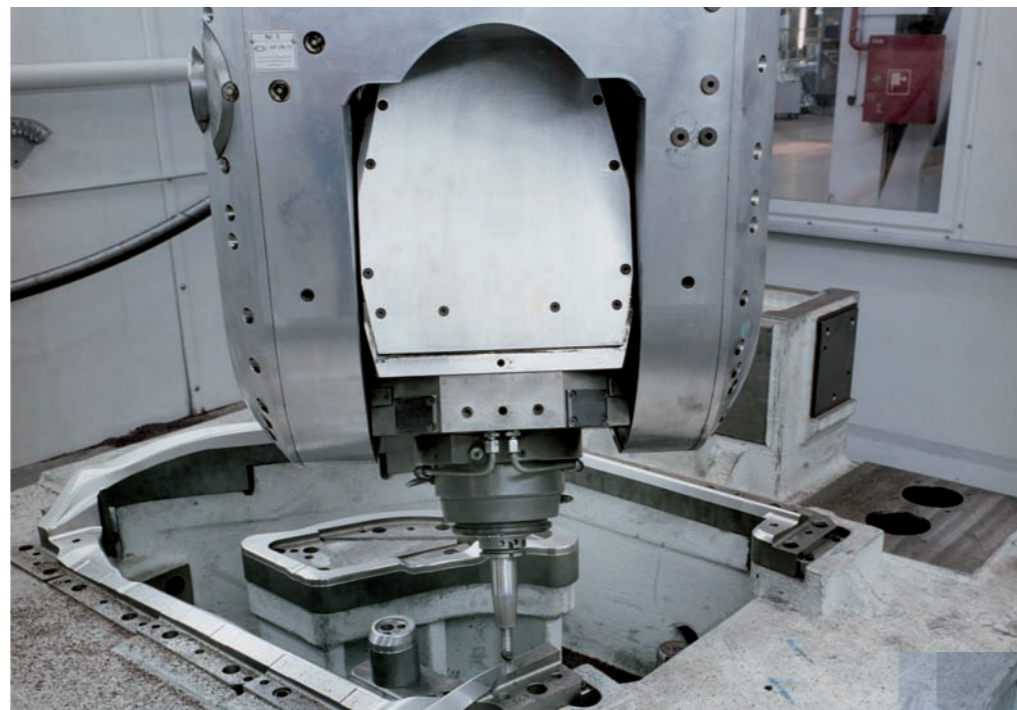
The workpiece – what will become a press tool – goes through every set-up and machining process on a single pallet, right from the incoming goods unit to the outgoing goods unit.
