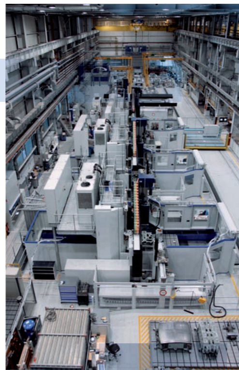
The pallet carriages link the individual work stations.
