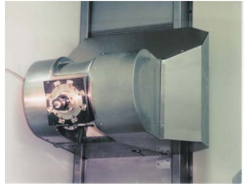
Tilting spindle of of the five-axis machining centre
