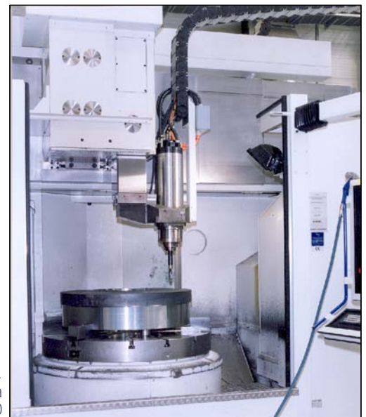
Drilling operation on a VCE 1600
