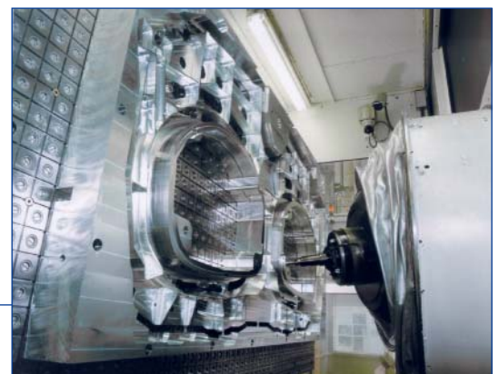
Processing of a structural component with Sprint Z3
